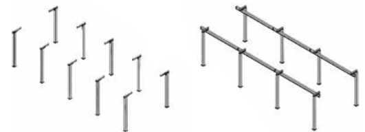
Lamp posts as freestanding support structure
